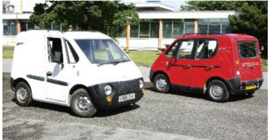
Stevens of Port Talbot's battery driven ZeCar® is designed for green city driving. It has five doors, is 3 metres long, and is 1.76 metres high. Top speed is 56 mph, has a range of up to 100 miles. It takes eight hours to top up the battery. Most important it costs just 2p a mile to run. On the road price is between £20 - 25,000. The makers claim it will pay for itself within three years.
