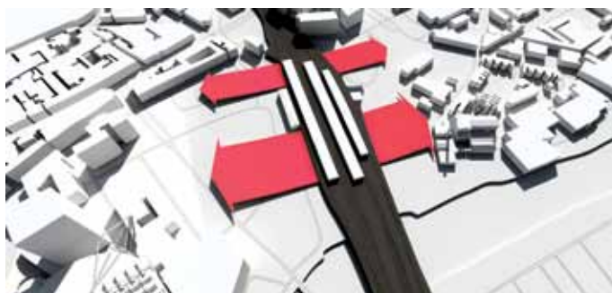
Figure 2: The current north-south connections through Cardiff station are limited to its ticketed concourse tunnel. If this were expanded, or if more of the fill under the station were removed, then the connectivity both spatially and visually would be substantial.
