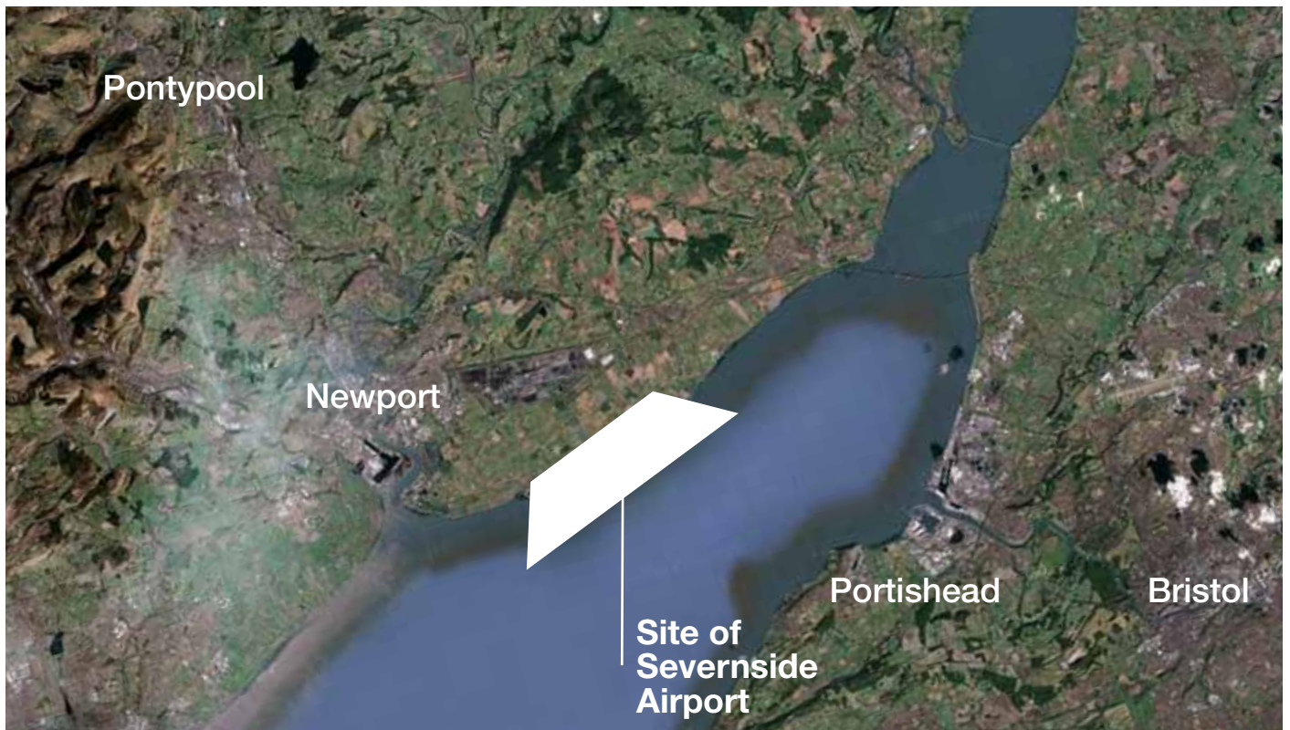
Map showing a potential site for Severnside Airport on the Welsh side of the estuary near Newport. One runway would be on shore with a terminal to the south. A second runway would be offshore parallel to the first. The airport would be served by road and rail from the M4 and the electrified Great Western Main Line.
